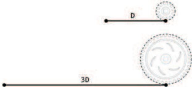
This means that the smaller gear must revolve three times in order for the large gear to revolve once; this results in the larger gear having (1/3) the rotational speed (RPM). Notice this is the inverse of the torque increase.
