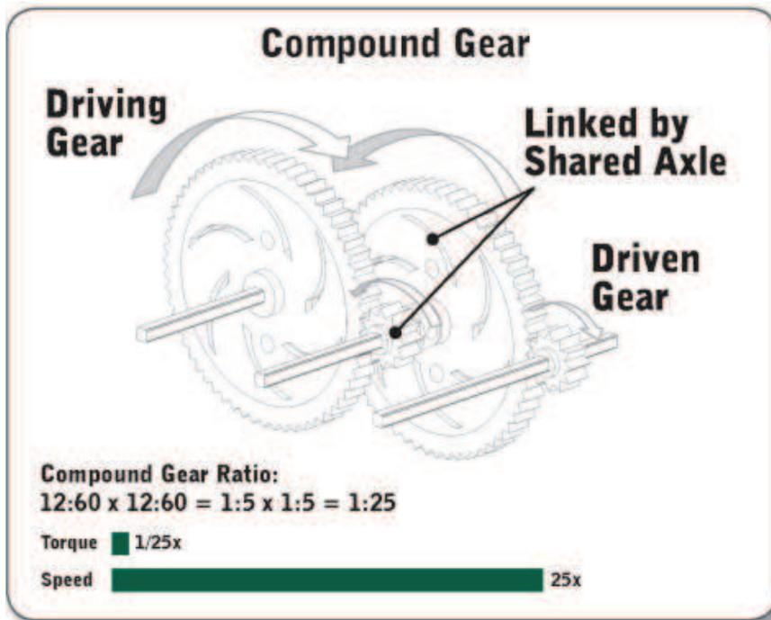
Compound gears allow configurations with gear ratios that would not normally be achievable with the components available. In the example above, a compound gear ratio of 1:25 was achieved using only 12 and 60-tooth gears. This would give your robot the ability to turn an axle 25 times faster than normal (though it would only turn with 1/25th of the torque)!
