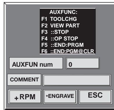
Figure G-15: To access this dialog box, press the + key (+ PGMSTOP) from the MDI Screen.
