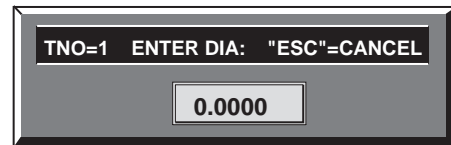
Figure G-4: TNO should equal your new Tool number. This box prompts you for the diameter of the Tool.
