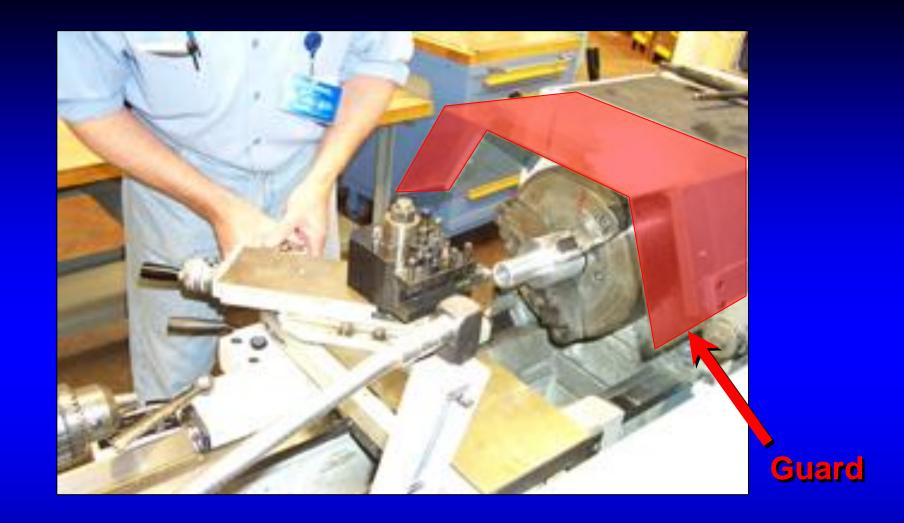
Always have the guard in place when the chuck is in motion.
