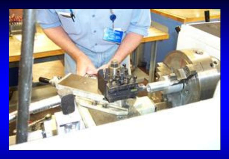
Move the tool bit a safe distance from the chuck when inserting or removing work.
