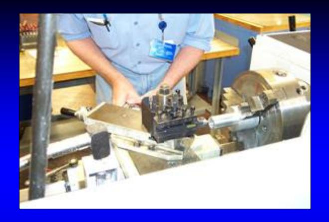
The lathe works tools into a workpiece which rotates on a spindle. It's useful for fabricating parts that have a circular cross section.
