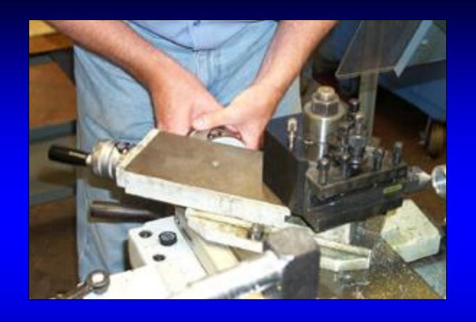
When operating the lathe, keep hands safely away from the tool and the rotating chuck.
