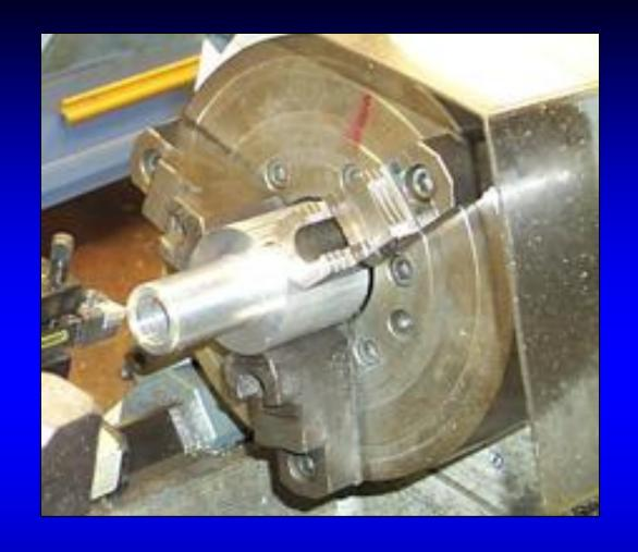
When operating the lathe, make sure the drive chuck is firmly tightened on the lathe spindle.
